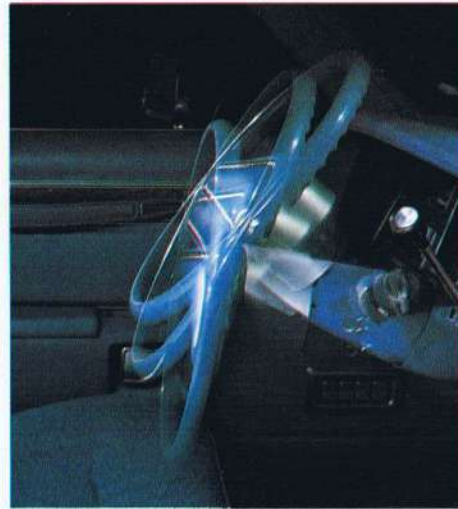
Tilt & Telescope Steering Column adjusts up and down, in and out, to suit each driver's comfort when entering or exiting.
