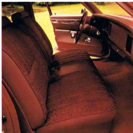
Standard Princeton cloth bench seat with vinyl trim and folding center armrest.
