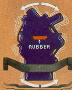
At the front, the Plymouth engine is suspended by this patented Floating Power mounting of live rubber inseparably bonded to steel.
