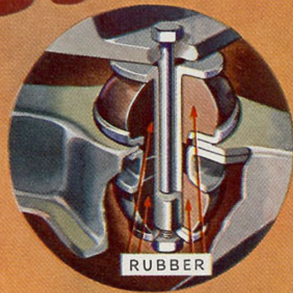
Spool-shaped mountings of live rubber, low at the rear of the Plymouth engine, absorb the gentle rocking motion of the engine.
