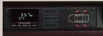
Acclaim LX has a "Traveler" mini trip computer and graphic message center that includes light outage indicators.
