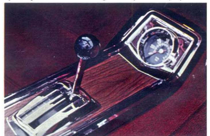
Console-mounted automatic transmission with Hurst linkage is a favorite with the sporty set.
