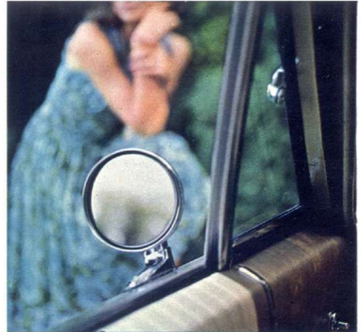
Aim outside mirror accurately and simply, without opening window, by adjusting control lever on inside of door panel.
