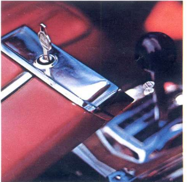
4-on-the-floor stick shift with Hurst linkage. Other features are standard from new crank-operated vent windows and special steering wheel with full horn
