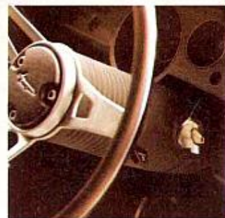
Anti-theft, column-mounted ignition switch.
