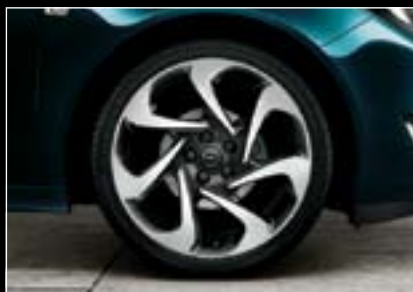
Jante alliage, 8,5 J x 20", 7 branches finition bicolore, pneus 245/35 R 20 (Q7R). 5
