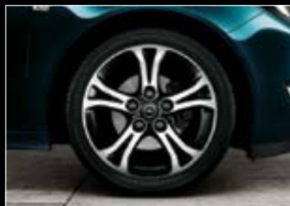
Jante alliage, 8 J x 18", 5 branches doubles triangulaires, finition bicolore, pneus 245/45 R 18 (Q7B). 7
