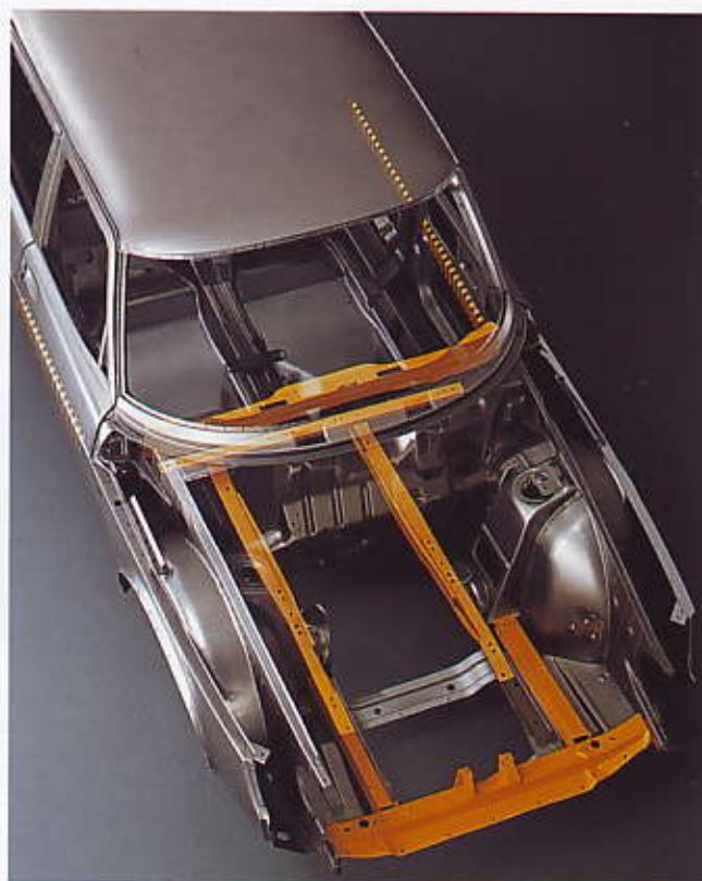
Crash members Members which transmit forces from a frontal collision to the wheel housings and arrest rearward movement of the engine.
