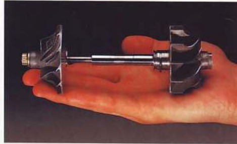
A turbine wheel—the foundation of turbo power.
