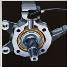
Wheel sensor A moisture-proof sensor at each wheel records the wheel's speed, which is registered by the ABS and TCS systems to immediately detect wheelspin or loss of traction.
