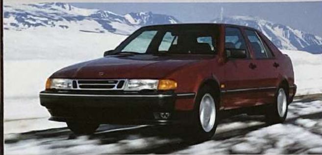
Keeping a grip on the road Saab's Traction Control System adjusts brakes (manual-transmission cars only) and throttle opening to address slippery road conditions.
