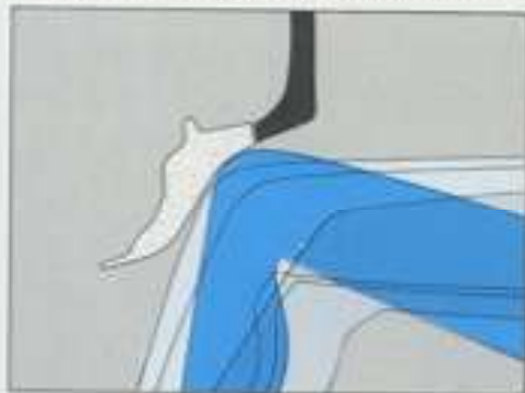
Impact-absorbing leg protector below the dash, designed to protect occupant's knees.
