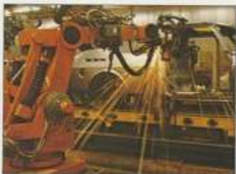
Advanced automatic welding contributes significantly to the overall sturdiness of the body.
