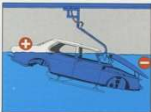
All Saab 900 cars are subjected to a comprehensive anticorrosion treatment at various stages during the manufacturing process.
