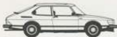
SAAB 900 TURBO, 3-DOOR. Turbocharged fuel-injection engine developing SAE net 135 hp (100 kW). 5-speed manual transmission or automatic transmission.
