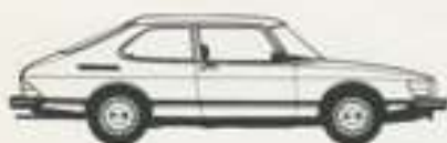
SAAB 900, 3-DOOR. Fuel injection engine developing SAE net 110 hp (81 kW). 5-speed manual transmission or automatic transmission.
