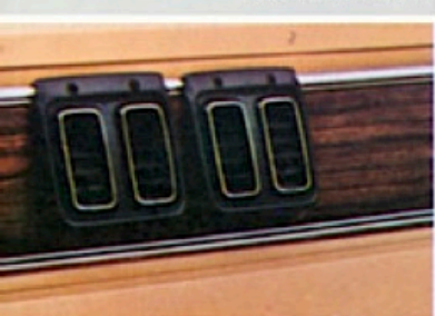
Rear Air Conditioning
