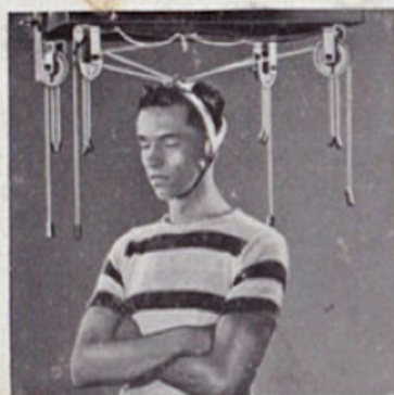
VISUAL ACUITY TEST —another one of the scientific tests to measure "auto fatigue"—records reduction in eye efficiency that results from driving strain. This test also supports the conclusions reached that drivers of the Dodge were less fatigued than after driving the competitive cars tested.
