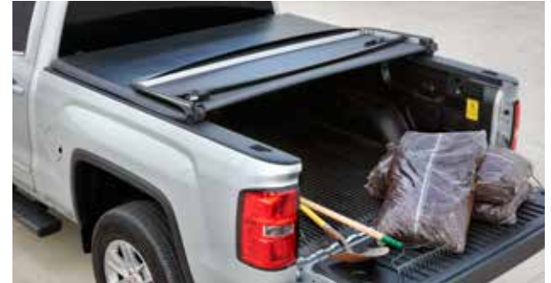
TONNEAU COVERS The soft cover shields cargo and easily rolls up to allow full access to the bed and is constructed with integrated crossbows. The hard cover is tri-folding and adds strong content protection and easy access to the cargo box.
