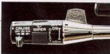
Electronic automatic speed control and intermittent windshield wipers (controls on multifunction switch)
