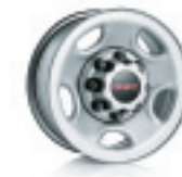
16-inch painted steel wheel, standard on WT models (QB5), available with chrome centre cap (P03)
