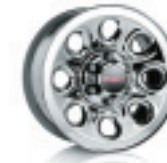
17-inch chrome-style steel wheel, standard on SLE and included on WT models with SL Package (PY9)
