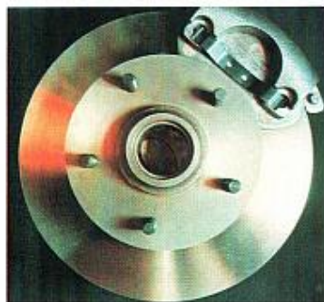
This page: Top: New steel rally wheel, 6" wide. Centre: Holden's economical smooth V8, 253 cubic inches, 185-hp. Left: New ventilated discs, 11" dia, 1" wide. Right: Reclining bucket seats. Facing page: Working area: the works.
