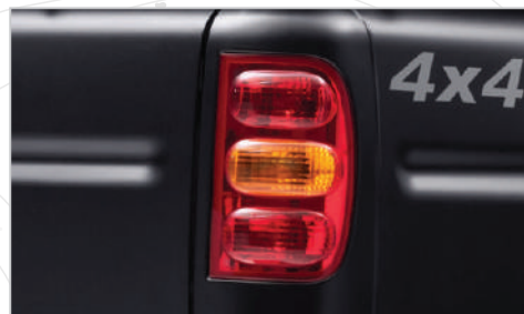
AUTOMATICALLY ACTIVATED HAZARD LIGHTS IN CASE OF SUDDEN BRAKING
