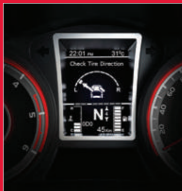
TYRE POSITION Displays tyre position to assist the driver when starting out.
