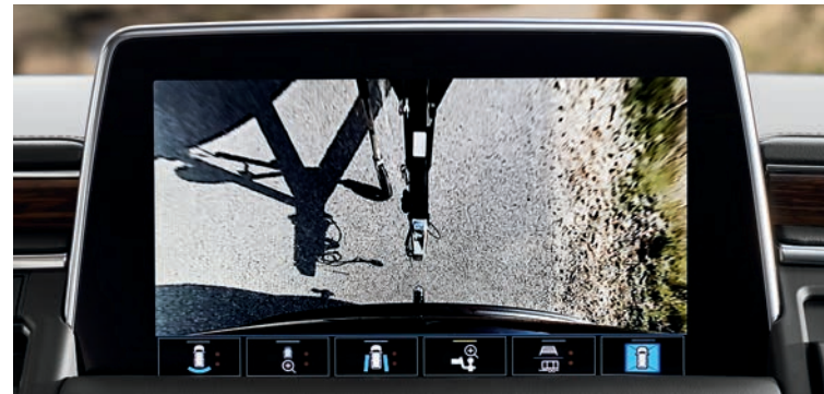
Hitch View Provides a close-up view of the receiver hitch to help with alignment when connecting to a trailer.
