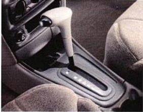
Console-mounted shifter for Malibu's standard 4-speed automatic transmission is anatomically shaped for a more comfortable, natural feel in your hand.
