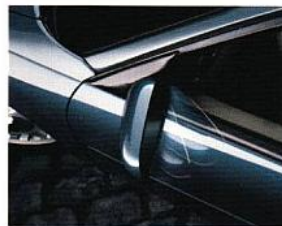
Malibu's dual outside rearview mirrors are designed to "break away" on impact to help protect pedestrians; they snap back into position undamaged.
