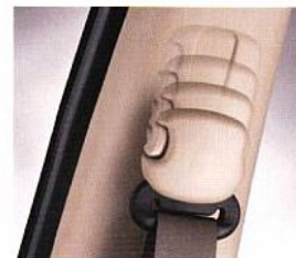
Because drivers and passengers come in all sizes, Malibu's front seat shoulder belts are height-adjustable to help keep everyone comfortable.
