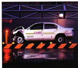
Designed-in crush zones at the front and rear of the car absorb crash energy to protect Malibu's occupants.
