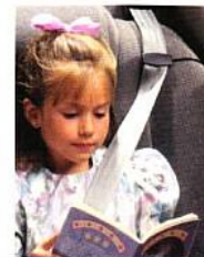
Special guides let you adjust the rear seat shoulder belts to make them more comfortable for smaller passengers.
