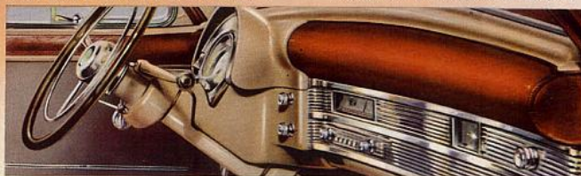
SAFETY CUSHION —Here's a safety feature of major importance! Front passengers, especially children, are given new protection against possible injury in event of sudden stops or collisions by the new sponge-rubber Safety-Cushion. It extends across the top part of the dash, and is upholstered in leather to match the interior.
