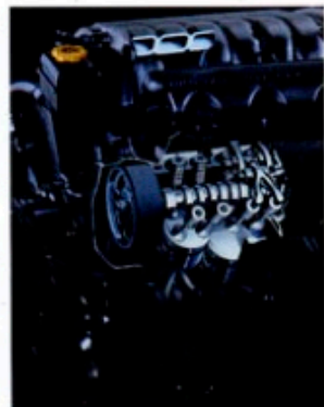
A 168-horsepower 2.5-liter SOHC SMPI 24-valve V6 power plant is available on LX and LXi.
