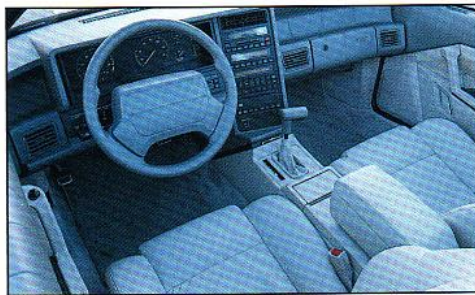
New seats (left) offer power lumbar support. Other comfort and convenience changes include a cup holder in console, easier access to interior cargo space. Dash has been changed so tach and speedometer readings keep pace with capacity of new engine
