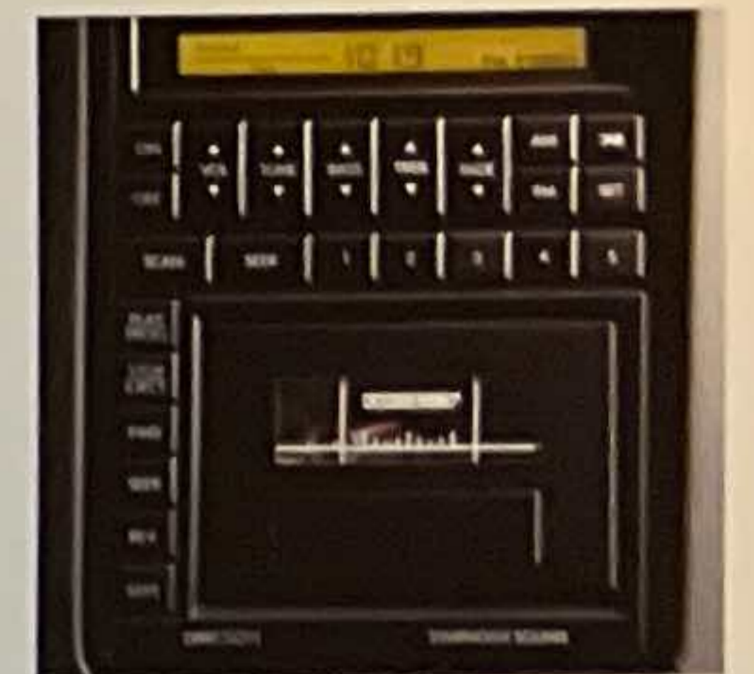
Allanté's Delco/Bose Symphony Sound System offers the sound balancing capabilities of a 32-band equalizer—automatically.
