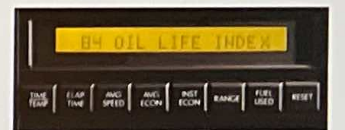
An oil life indicator suggests optimal oil change intervals.
