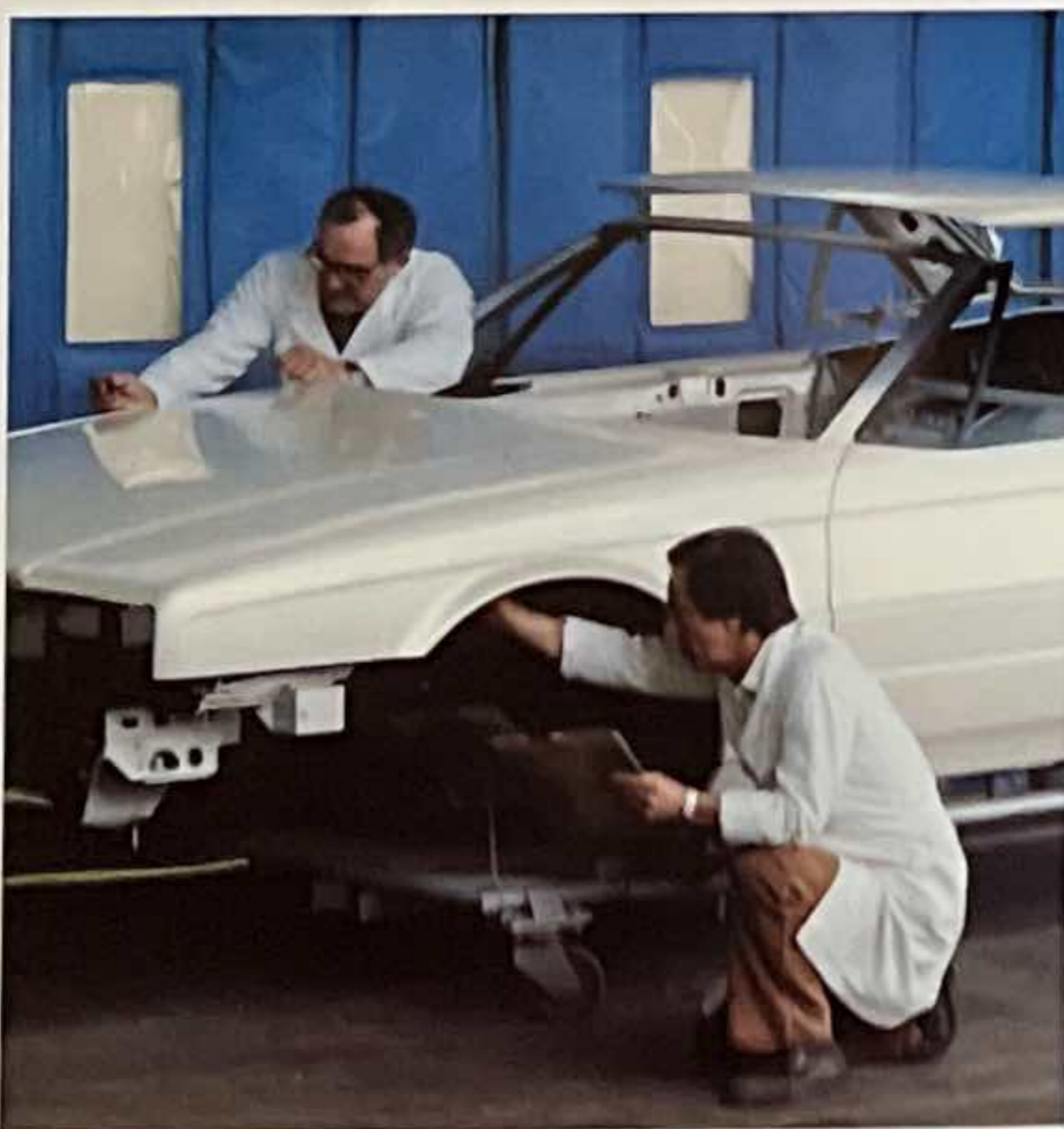
Doors, hood, rear deck lid and fenders are handfitted by skilled Italian craftsmen.
