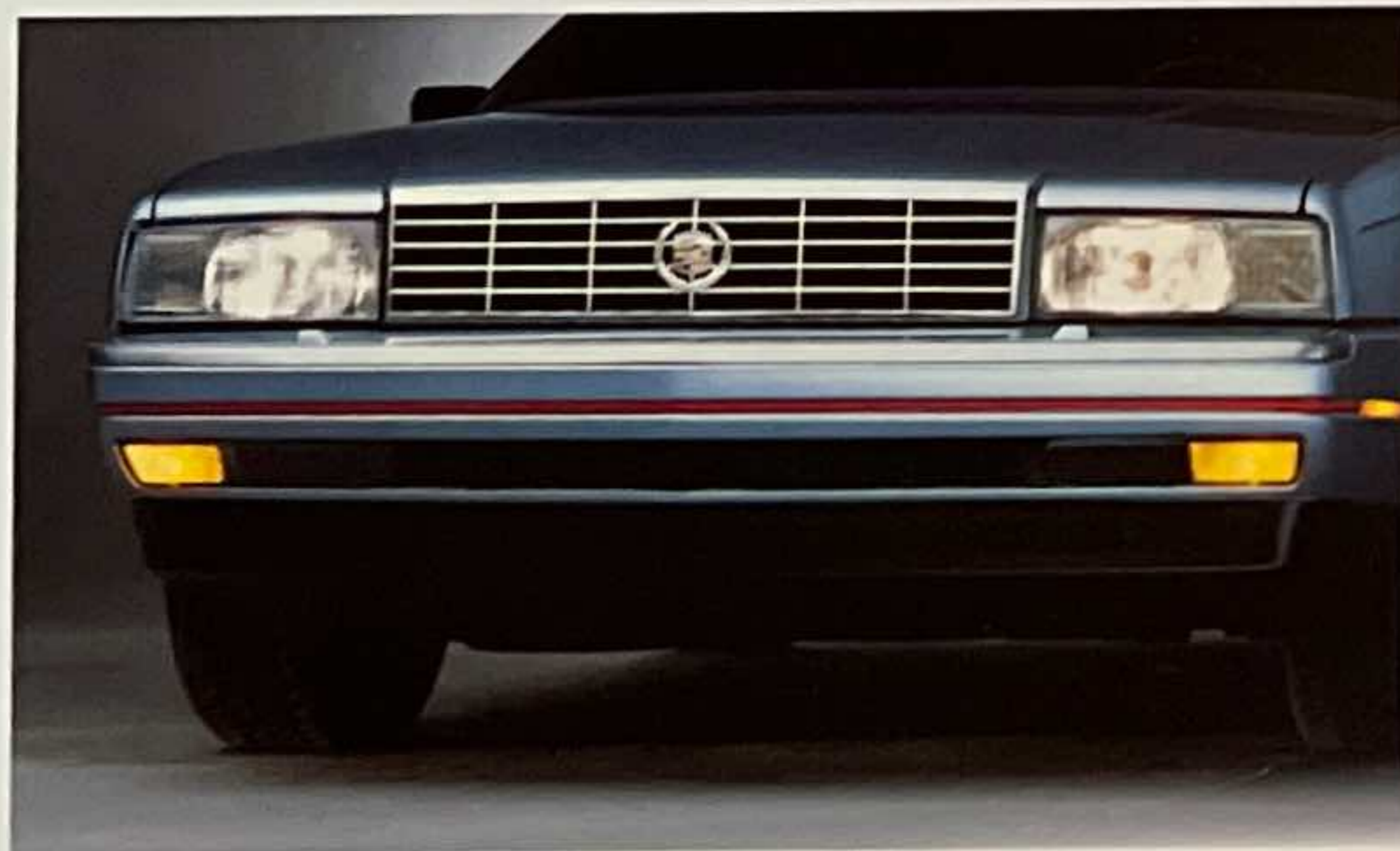
Allanté's exclusive multiplex wiring acts as a back-up system. It allows a non-functioning lamp to be substituted by a nearby lamp until replaced.
