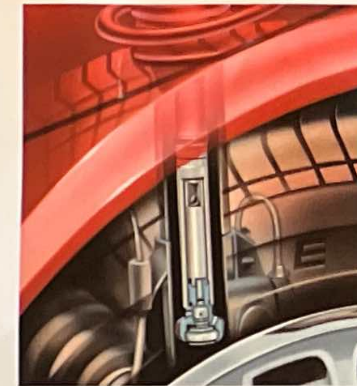
Strut damping is adjusted automatically based on vehicle speed and brake input to help provide optimum ride and handling at any speed.
