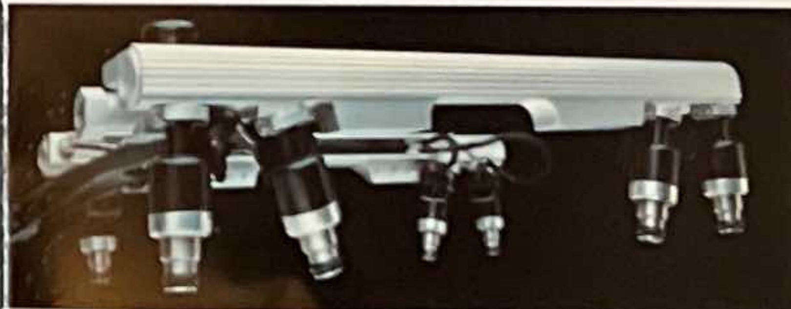
A staged, twin-throat throttle body with sequential-port fuel injection assures precise fuel delivery timing.
