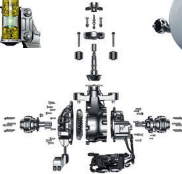
ELECTRONIC LIMITED-SLIP DIFFERENTIAL The CTS Vsport includes an electronic Limited-Slip Differential (eSLD) that uses vehicle sensors and driver inputs to determine the optimum amount of engagement for the conditions. This optimized torque split between the rear wheels allows for precise steering feel, enhanced stability, and maximum traction through corners.
