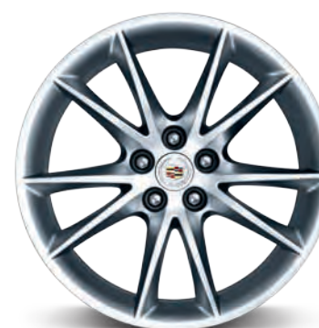
20" CAST-ALUMINUM WITH PREMIUM MULTI-COAT PAINTED FINISH PREMIUM COLLECTION OPTION (INCLUDED ON VSPORT PREMIUM); INCLUDES P245/40R20 ALL-SEASON TIRES 1
