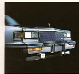
Front Air Dam with Integrated Front Fog Lamps.
