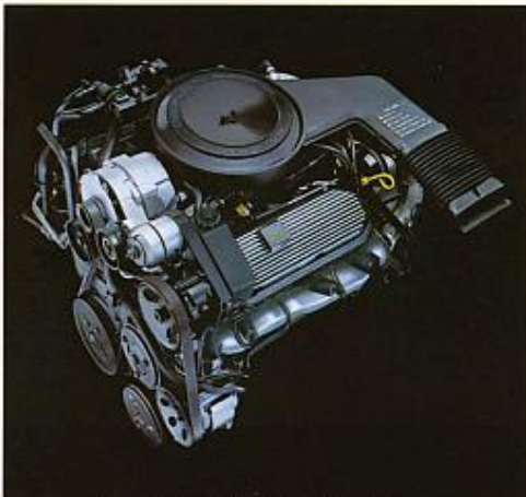
Transverse-Mounted HT 4100 (4.1 Liter) V8 with Digital Fuel Injection.
