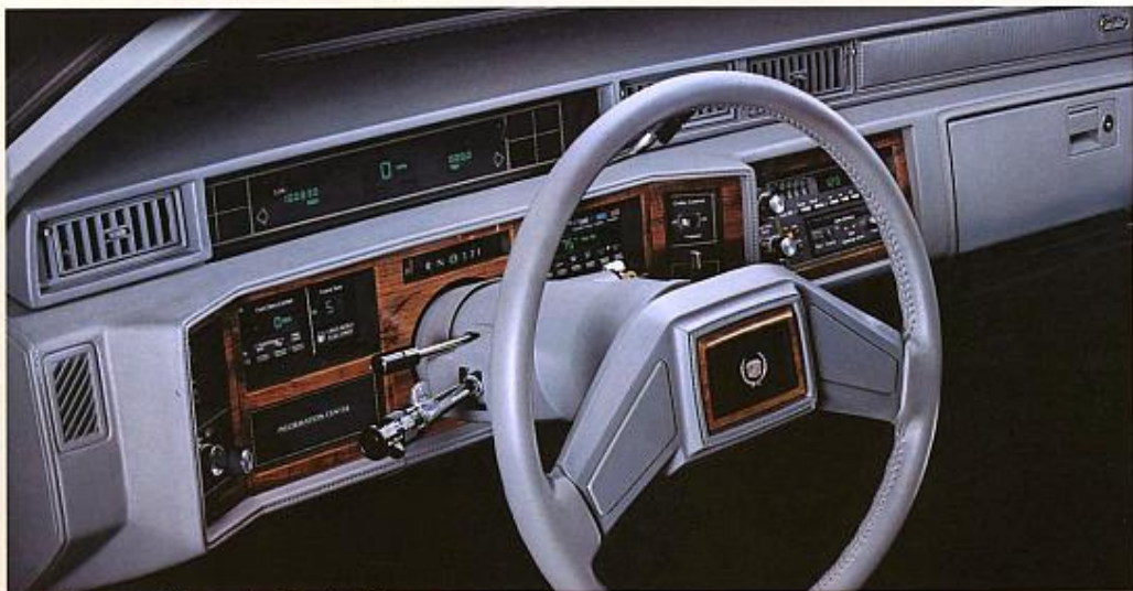
Digital Instrument Cluster, a New Standard Feature.
