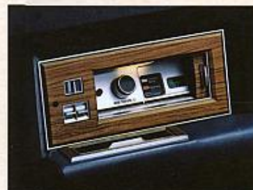
Rear Electronic Climate Control Panel with Outside Temperature Display.
