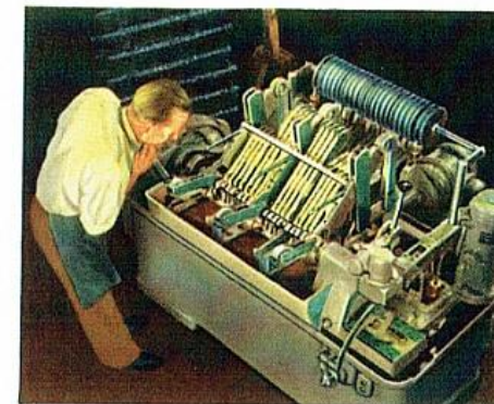
Developed for, and first used by, Cadillac, this remarkable machine polishes all the lobes of the camshaft at once to a four-millionth inch finish. A special testing device maintains a constant check on accurate machine operation by measuring these slight irregularities on the cam surface.
