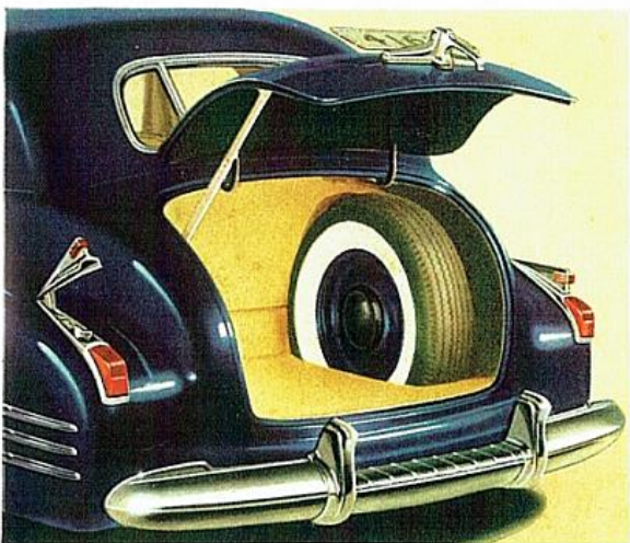
Closed sedan models carry the spare wheel mounted upright on the side of the spacious, automatically lighted rear compartment. On all Cadillacs the gas tank filler cap is concealed under the left tail light.
