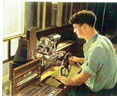
In a secluded booth, every transmission gear is checked for exactness of tooth contours. Johansson gauge blocks, shown in the foreground, maintain a constant check on the accuracy of the production gauge. They are the basis for the matchless precision of Cadillac manufacturing.
