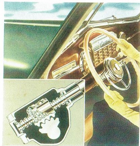
The ball bearing steering gear was pioneered by Cadillac. This important new advancement, shown in inset, is not only stronger than conventional assemblies, it also gives Cadillac cars unexcelled steering ease.
