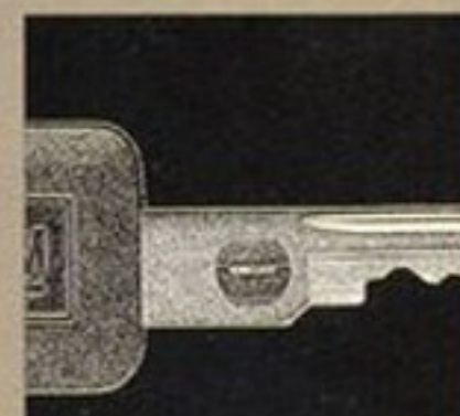
A specifically coded resistor in the key helps PASS-Key® II prevent unauthorized starts, while a full-feature theft-deterrent system helps prevent vehicle entry for SSEi.
