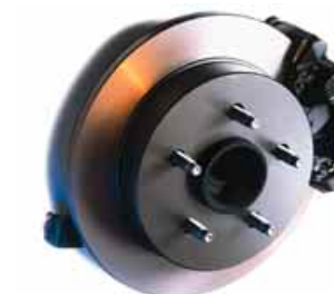
Standard four-wheel discs with anti-lock braking system (ABS) incorporate front ventilated front discs that rapidly dissipate heat. The brakes also emit a warning sound when pads need to be replaced.
