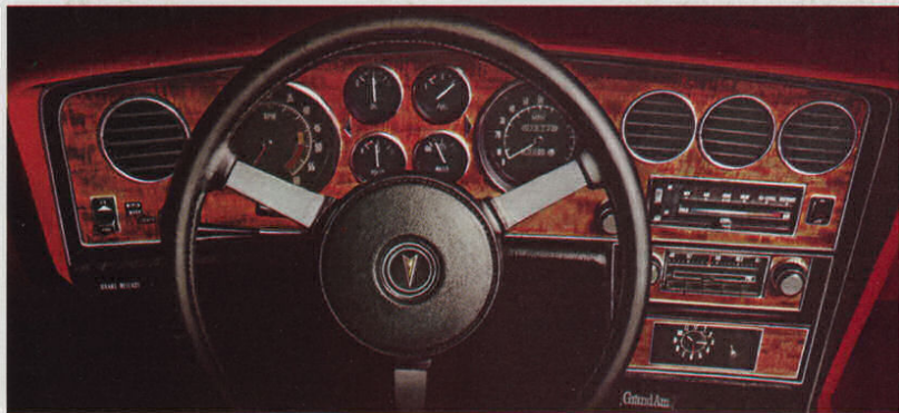
Grand Am instrument panel with standard rally gauge cluster and available tachometer.
