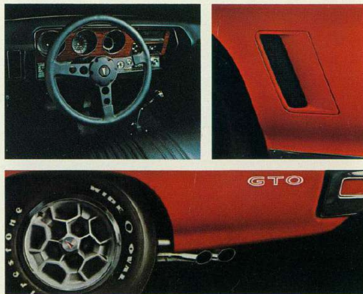
Above: optional Formula steering wheel, standard front fender air extractors, optional honeycomb wheel, standard side exhaust outlets.
