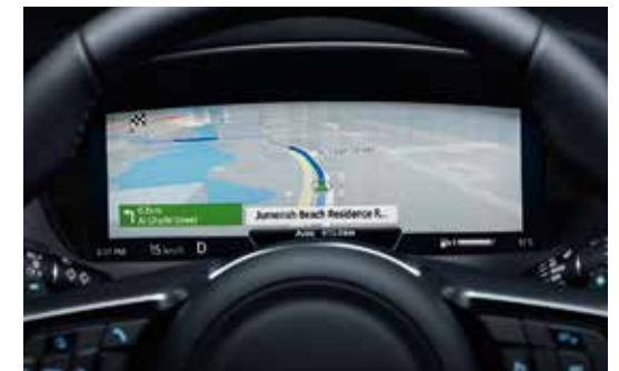
12.3 inch Instrument Panel Display with full screen 3D Map View
