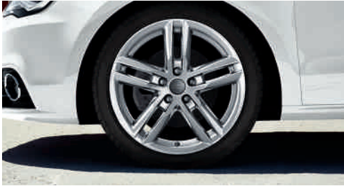
Audi exclusive cast aluminium wheels in 5-twin-spoke design size 7.5 J x 17 with 215/40 R 17 tyres. From quattro GmbH
