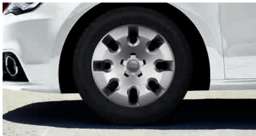
Steel wheels with full wheel covers size 6 J x 15 with 185/60 R 15 tyres (exclusively for 1.2 TFSI Attraction); size 6.5 J x 15 with 205/55 R 15 tyres
