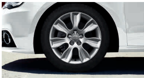
Cast aluminium wheels in 7-arm dynamic design size 7 J x 16 with 215/45 R 16 tyres (also available with run-flat tyres)
