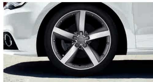
Cast aluminium wheels in 5-arm design with decorative elements, size 7.5 J x 17 with 215/40 R 17 tyres
