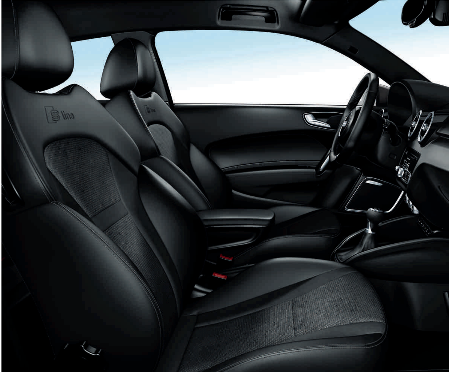
Sports seats in sprint cloth/leather, black, with S line embossing and contrasting stitching, black centre console in mono.pur, air vent sleeves in high-gloss black. (The image shows the Audi A1.)
