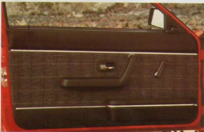
Fabric lining on doors.
