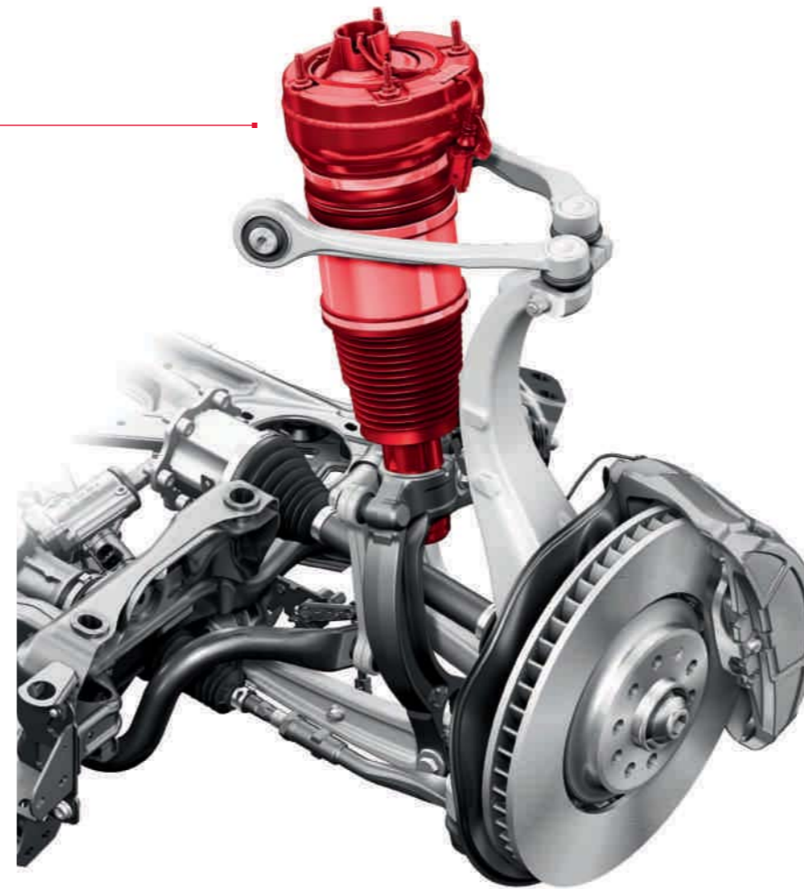
The infinitely variable damping adjusts itself automatically to every driving situation in fractions of a second. Even with asymmetrically distributed loads, the vehicle remains in a level position thanks to continuous ride-height regulation. Drivers can determine how dynamically they want to travel and what character their Audi should adopt. Different modes are available to the driver and can be selected using the Audi drive select system.
