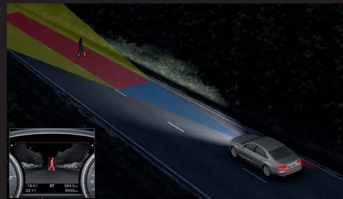
Should the system detect an imminent collision, the marking turns from yellow to red and a warning tone will sound.
