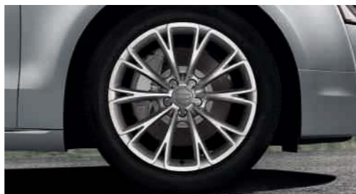
Cast aluminium wheels in 10-spoke Y design, partially polished, size 9 J x 19 with 255/45 R 19 tyres
