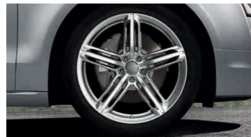
Audi exclusive cast aluminium wheels in 5-double segment spoke design, size 9 J x 20 with 265/40 R 20 tyres
