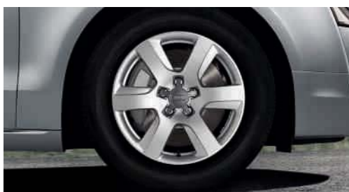
Forged aluminium winter wheels in 6-arm design, size 7.5 J x 17 with 235/60 R 17 tyres, suitable for snow chains, permissible top speed 210 km/h
