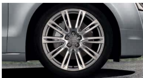
Forged aluminium wheels in 10-parallel spoke design, partially polished, size 9 J x 20 with 265/40 R 20 tyres
