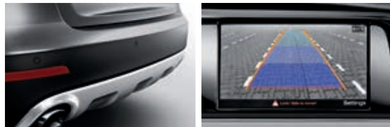
Parking system plus with rear acoustic sensors Parking system plus with rear view camera
