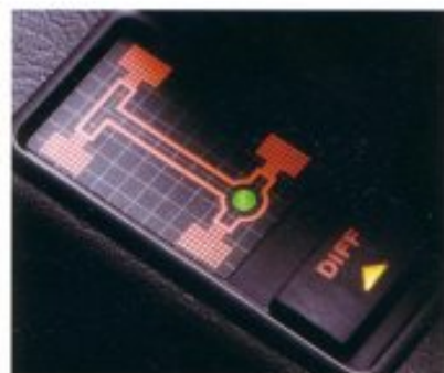
Switchable rear differential lock aids traction from standstill.
