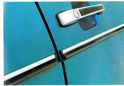
The trim around the car's waistline has a rubber strip to protect the paintwork
