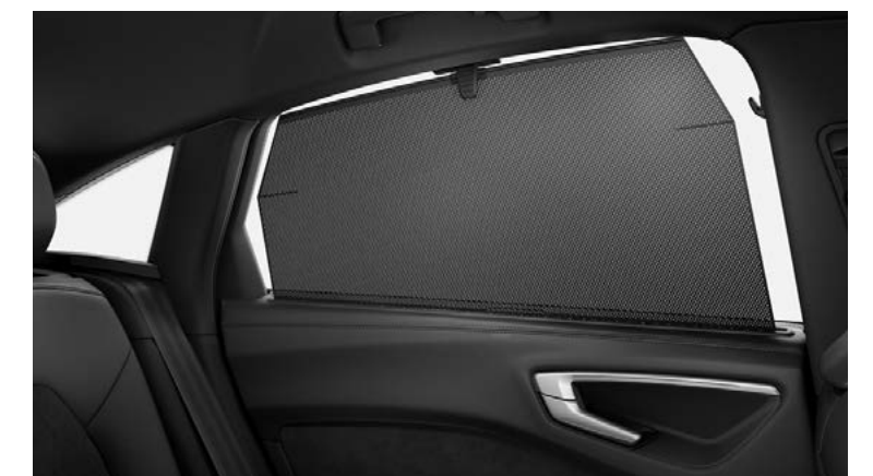
Stores pare-soleil manuels [3Y4]
