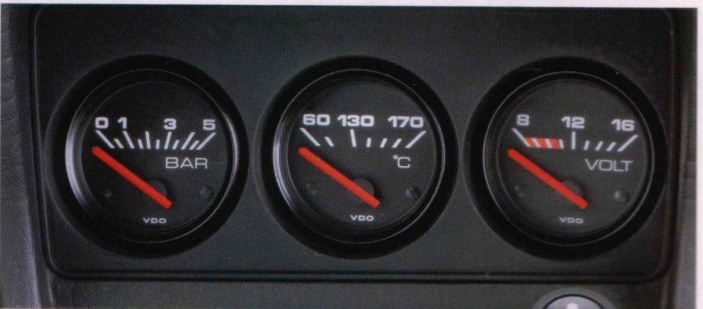
Oil temperature, oil pressure and voltmeter (GT).
