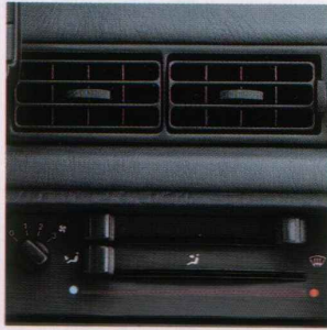
Heating and ventilation system with 3-speed fan.
