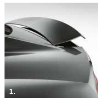
Main image. R8 V10 in Daytona grey, pearl effect (6Y). 1. Retractable rear spoiler. 2. Door sill trims with aluminium inlays and R8 logo. 3. R8 3-spoke, flat-bottomed, multi-functional, performance leather steering wheel with 2 operating satellites. 4. Deluxe 1-zone climate control.
