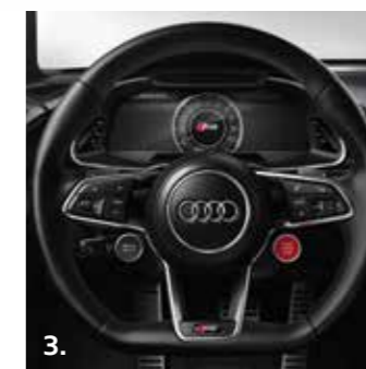
Main image. R8 V10 in Daytona grey, pearl effect (6Y). 1. Retractable rear spoiler. 2. Door sill trims with aluminium inlays and R8 logo. 3. R8 3-spoke, flat-bottomed, multi-functional, performance leather steering wheel with 2 operating satellites. 4. Deluxe 1-zone climate control.
