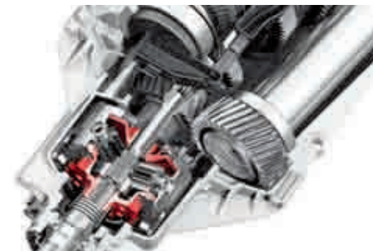
The crown gear centre differential has disc sets to achieve higher blocking factors. This allows up to 85% of the drive torque to be distributed to the rear axle and up to 70% to the front axle.
