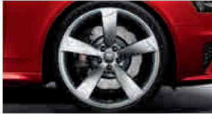
Cast aluminium wheels in 5-arm rotor design size 9 J x 20 with 265/30 R 20* tyres
