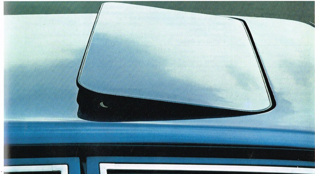
Steel sliding sunroof – open (standard on the CD).
