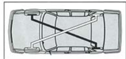
The diagonally linked dual circuit braking system. The two braking circuits on the Audi 200 are diagonally linked. If one circuit fails, the brakes will still work on one front wheel and on the diagonally opposite rear wheel. The braking power is evenly distributed between front and rear, with 50% of the braking effect on each axle.
