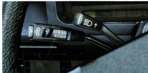
Automatic cruise control. (Standard equipment on the 200 ST, available as an optional extra on the 200 SE.)
