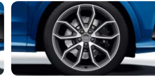
Cast aluminium wheels in 5-twin-spoke V design in matt titanium look, gloss turned finish 2 size 8.5 J x 20 with 255/35 R 20 tyres 1
