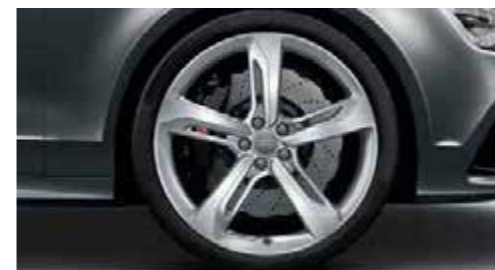
Cast aluminium wheels in 5-spoke blade design size 9 J x 21 with 275/30 R 21 tyres*
