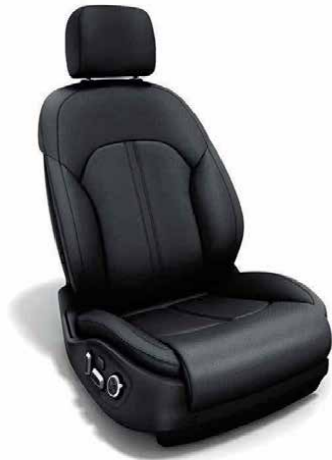
Comfort seats, front, with memory function with electric adjustment of seat height, fore/aft position, backrest angle, seat angle and thigh support; pneumatic adjustment of seat and backrest side bolsters as well as lumbar support; manual adjustment of head restraint height and clearance, as well as seat belt height; including memory function for driver and front-passenger seat, electric steering wheel adjustment and exterior mirrors; optional seat ventilation, front (The image shows comfort seat, front, with memory function and seat ventilation, front, in perforated Valcona leather, black.)
