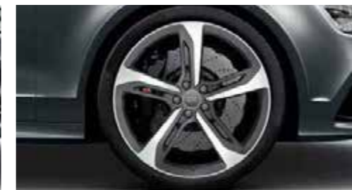
Cast aluminium wheels in 5-spoke blade design in matt titanium look, high-gloss turned finish size 9 J x 21 with 275/30 R 21 tyres*
