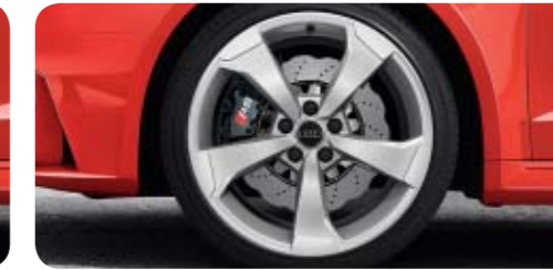
Cast aluminium winter wheels in 5-arm rotor design size 8 J x 19 with 235/35 R 19 winter tyres 1 , can be fitted with snow chains, permissible top speed 240 km/h
