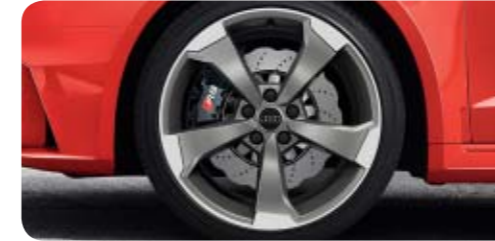
Cast aluminium wheels in 5-arm rotor design in titanium look, gloss turned finish 2 size 8 J x 19 with 235/35 R 19 tyres 1
