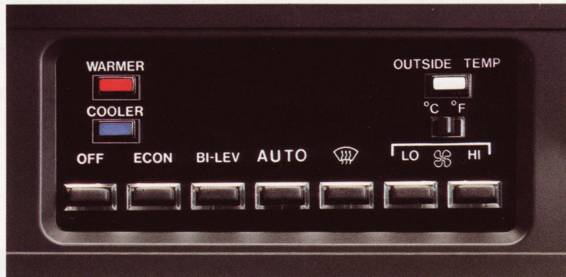
Control panel for the fully-automatic air-conditioning unit.
