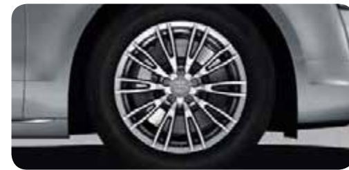
Cast aluminium wheels in 10-spoke V design size 8 J x 18 with 235/55 R 18 tyres*
