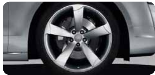
Audi exclusive cast aluminium wheels in 5-arm rotor design size 9 J x 21 with 275/35 R 21 tyres*. From quattro GmbH
