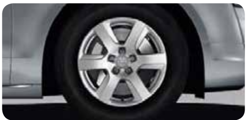
Cast aluminium winter wheels in 6-arm design size 7.5 J x 17 with 235/60 R 17 tyres*, permissible top speed 210 km/h, can be fitted with snow chains
