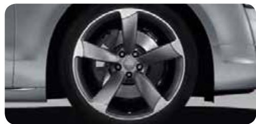
Audi exclusive cast aluminium wheels in 5-arm rotor design matt titanium look, gloss turned finish size 9 J x 21 with 275/35 R 21 tyres*. From quattro GmbH
